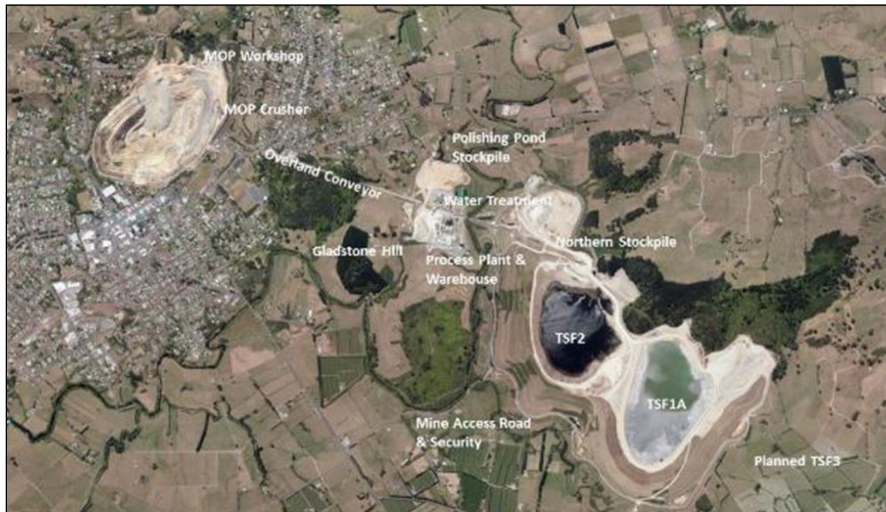
Figure 1-5: Waihi Existing and Planned Infrastructure
